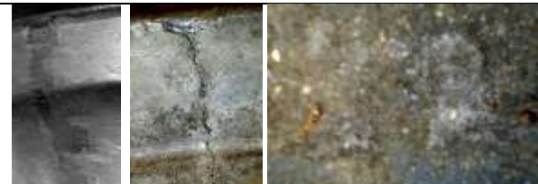
There was a repaired casting fault or even later split from the front central rim downwards for 4cms - there were no marks in the base.
