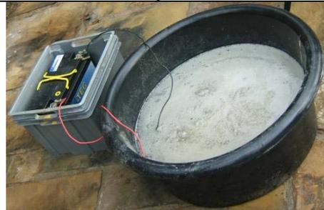
This shows a similar set up for cleaning plates. The negative is attached to the plate and the positive to a stainless mesh disc placed free of the plate and above it in the water. This trying to clean a 20" plate. The black tub is a man made garden pool liner.
