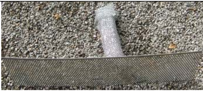
This shows the probe made out of rolled stainless wire mesh.
