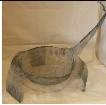
A home made wire mesh framework to stand in the bowl and over it whilst not touching it I attached the positive to the tail and the negative to the bowl.
