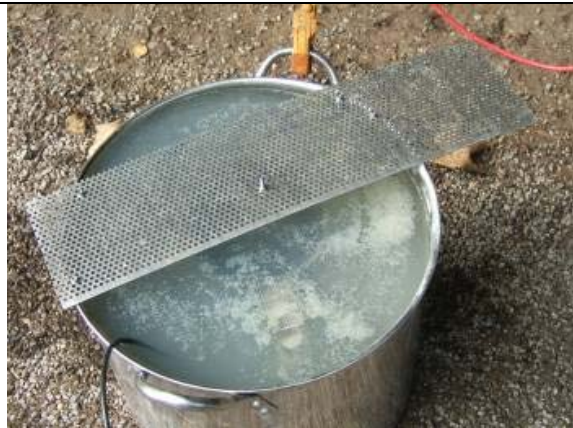
You can see the process progressing in the bubbling in the bucket. The grid across the top is shown below with an attachment to go down into the measure to be cleaned. This 'probe' must not touch the base of the measure or the sides – some use say a stainless steel fork. hung there.
