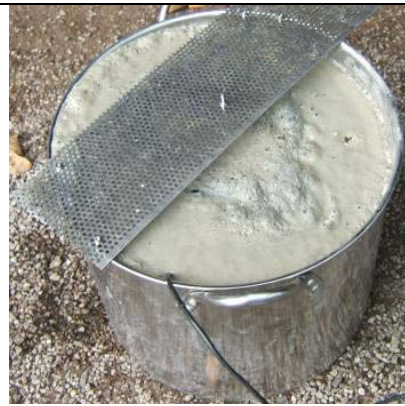
As you can see the 'froth' on the top – I used perhaps too much washing soda which releases hydrogen which hovers over the top of the bucket.
