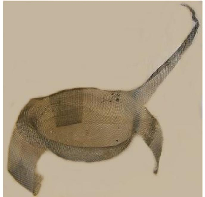
1. Framework made from a fine woven stainless steel mesh to follow the contours of a bowl I was cleaning.
