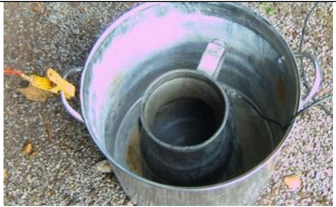
Showing the positive terminal clip attached to the pan handle and the negative clip to the piece to be cleaned with the measure stood on the rubber mat before the addition of the water or electrolyte solution (water they say will do it alone without washing soda).
