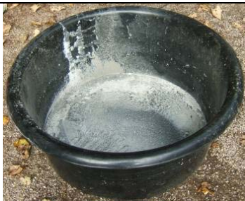
After the cleaning there can be a lot of oxide remaining in the container. If this is dried and ground down in a mortar it can be made use of in other repairs as it is simply pewter (or pewter oxide) dust.
