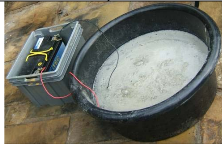
As you can see the 'froth' on the top – I used perhaps too much washing soda which releases hydrogen which hovers over the top of the bucket.
