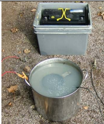
Cleaning underway (almost – just the leads to be connected to the battery). The battery is put into a plastic carrying box as battery acid splashes about. yes it might destroy the container but it saves your clothes!
