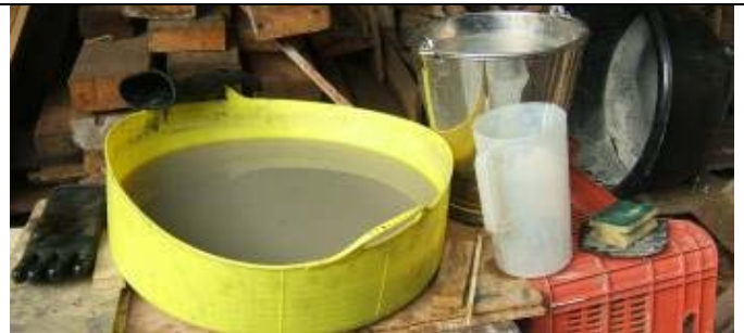
The purpose of this photo is to show some of the commonly found kit that can be used. A flat garden or plasterers trug (yellow) can clean plates up to 16" in the largest size I found. Rubber gloves – well electricity and some heat! Stainless steel bucket, plastic water jug, kitchen pad (keep it softer rather than hard)
